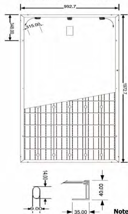
DIMENSION OF PV MODULE
