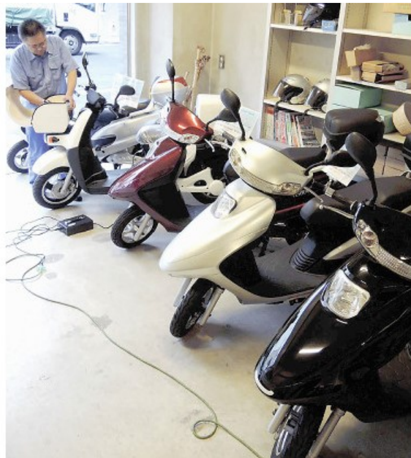
Electric motorbike can be charged without special charging equipment. Generally, an electric motorbike can run 30 ~ 60 km after fully charged. Cost efficiency is much higher than motorbikes that run on gasoline. Source: Yomiuri online
