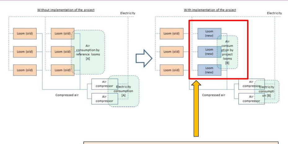
Project loom can reduce CO<sub>2</sub> emission compared with the reference loom by saving the load of air compressors through the air saving technology,
